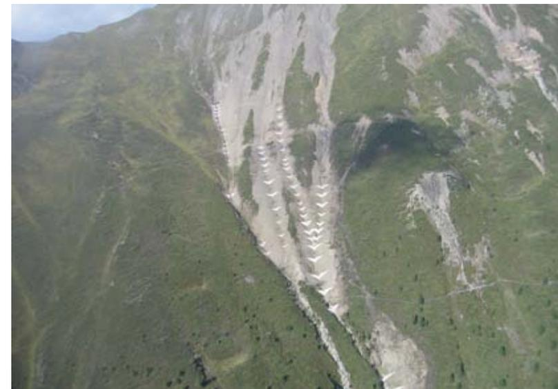
Fig. 2: Erosion areas in the area of the Steggraben – project measures – and consolidation of the stream bottom and the seeding and greening of open areas.
